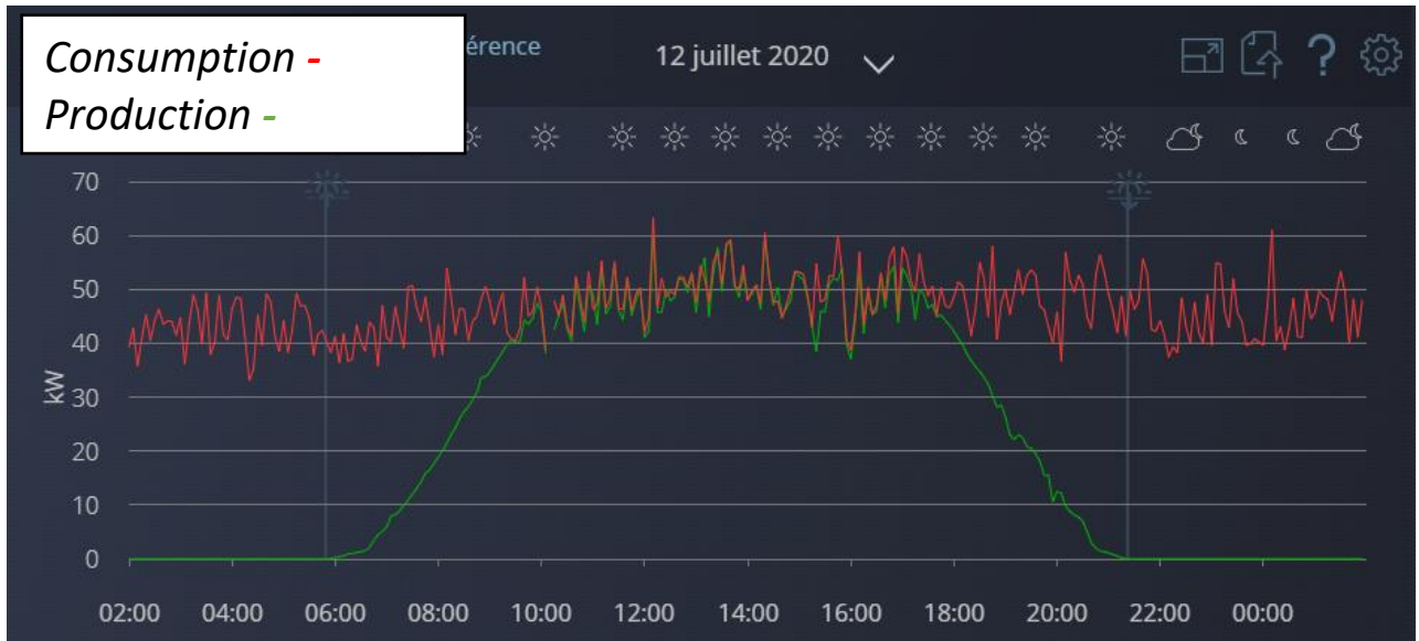
Figure 6.2: Example of self-consumption PV plant
